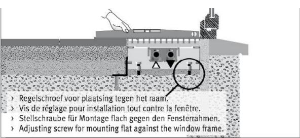
Levelling of the trench heater is achieved using the jacking screws 1. Once a level trench is achieved, the "L" profile bracket 2 can be fitted in the required location and tightened to the side of the trench. The base of the "L" profile can now be fastened to the floor (due to the wide variety of floors, Jaga do not supply these fasteners).
